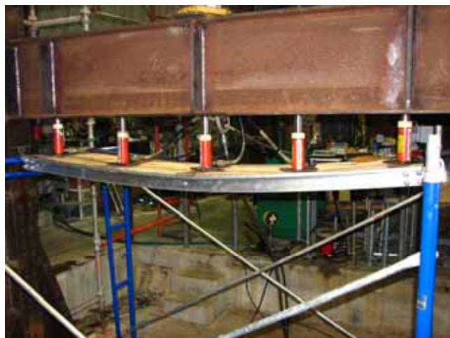
Uniform load application. Right photograph shows load at 11,000 lbs.
