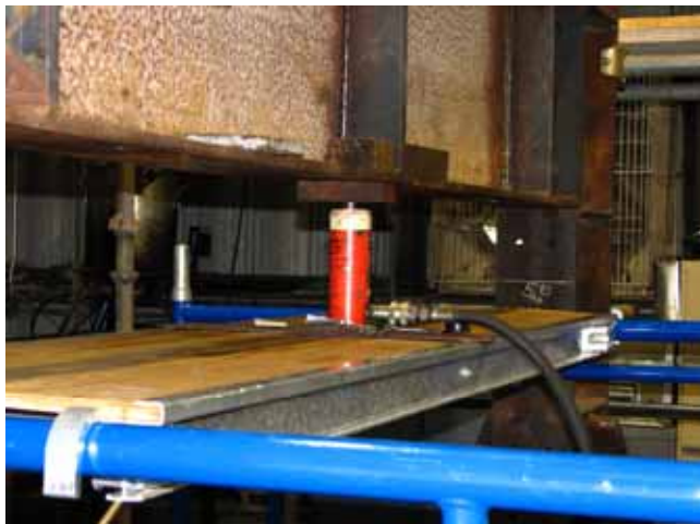
Point load application. Right photograph shows load at 2,430 lbs.
