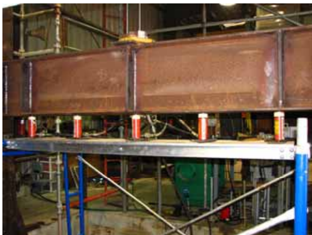
Uniform load application. Right photograph shows load at 11,000 lbs.
