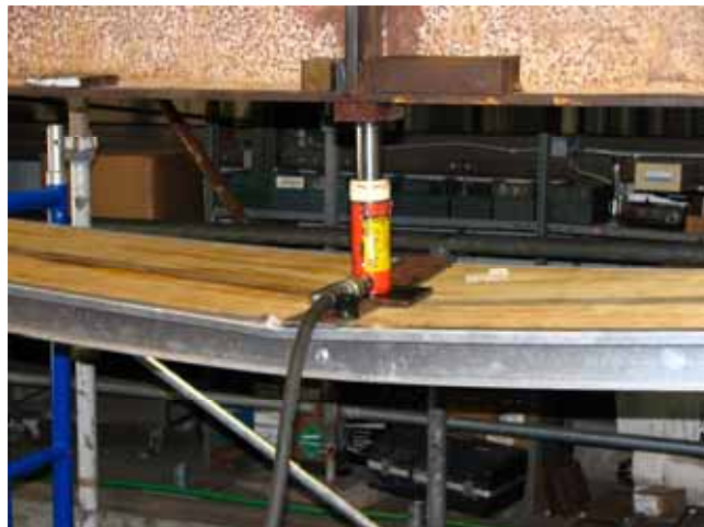
Point load application. Right photograph shows load at 2,430 lbs.
